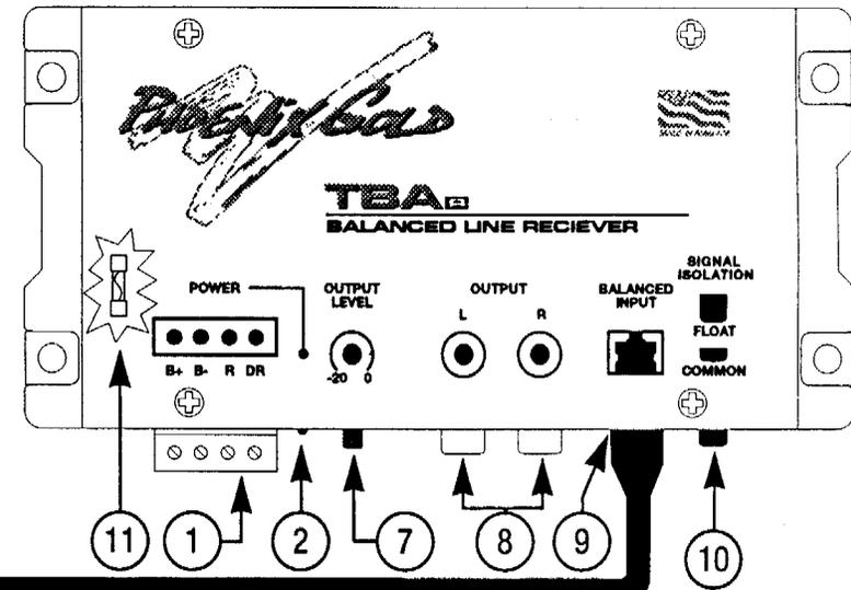
1. **Quick Disconnect Power Plug:** This connector is easily unplugged for servicing wiring connections and contains the following terminals:
